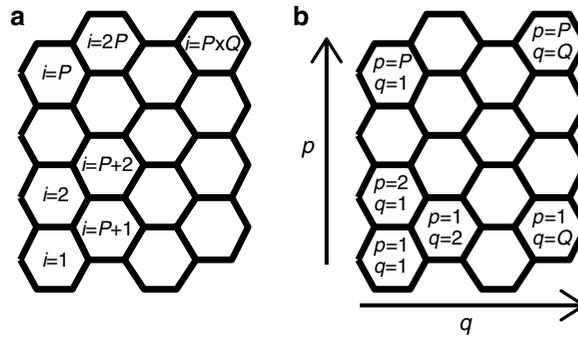
**Fig. 2** Labeling schemes in a regular hexagonal cell lattice. **(a)** One index labeling scheme. **(b)** Two indices labeling scheme. Having two indices per cell facilitates the computation of the neighboring cell indices and the implementation of the periodic boundary conditions
